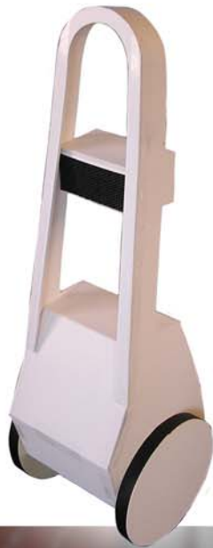
Early mock-ups Volume studies were completed to quickly evaluate scale and proportions.
